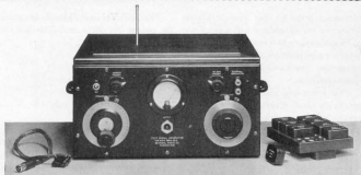
FIGURE 1. A TYPE 604-B Test-Signal Generator showing the smallest of the three rod-type antennas. Voltage can also be delivered to the receiver under test by means of the cable, the jack for which is on the panel. The coil-mounting rack and the 13 coils supplied with the instrument can be stored in a compartment inside the cabinet.
