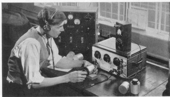
FIGURE 5. Inspecting TYPE 653 Volume Controls for noise. Every General Radio volume control is individually tested for noise, attenuation, and impedance, as well as the usual mechanical inspection
