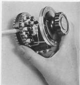
FIGURE 2. This unique construction guarantees ruggedness and a flat frequency characteristic for all settings over the entire attenuation range. Note that the shaft is insulated and that the frame is at ground potential
