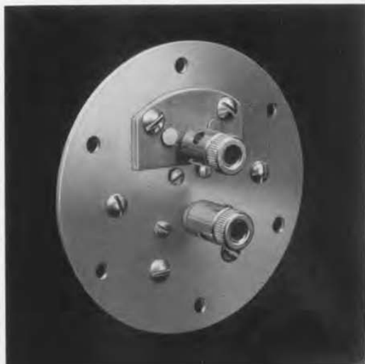
FIGURE 4. Outside view of the voltage standard of Figure 2, indicating shielding of the output terminals from the ground leads. The standard was made as a detachable unit so that it could be used in several assemblies
