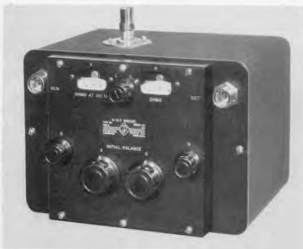
Figure 4. View of the engineering model of the V-H-F Bridge with coaxial adapter installed on the unknown terminal at the top of the cabinet. Panel size is approximately 11 x 9 inches. Production model has a larger ground plate around the unknown terminal and is equipped with carrying handles.
