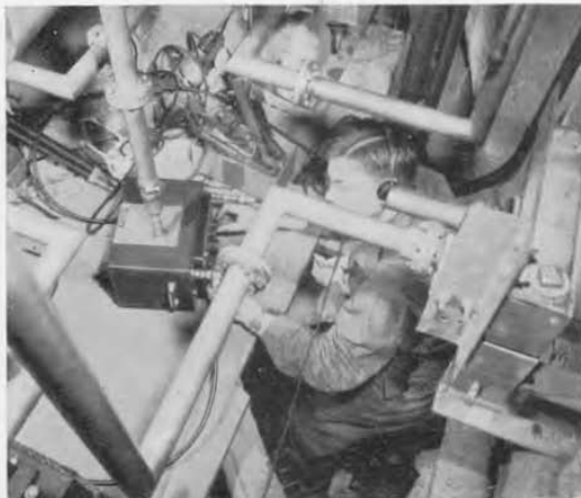
Figure 1. Ogden Prestholdt, CBS engineer, using the V-H-F Bridge to measure the new antenna of WCBS-TV, on the Chrysler Building. Some of the results of the measurement are shown in Figures 7 and 8, page 5.
