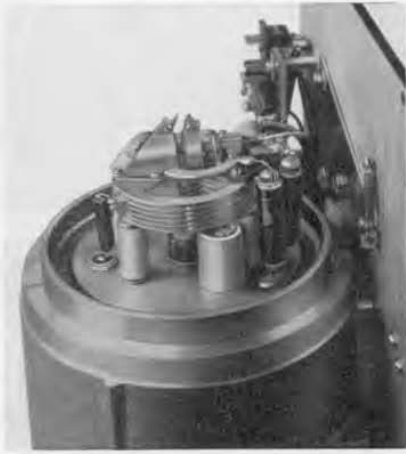
Figure 3. View of the oscillator portion of the U-H-F Unit, with cover removed from casting to show tube, butterfly, and attenuator input.
