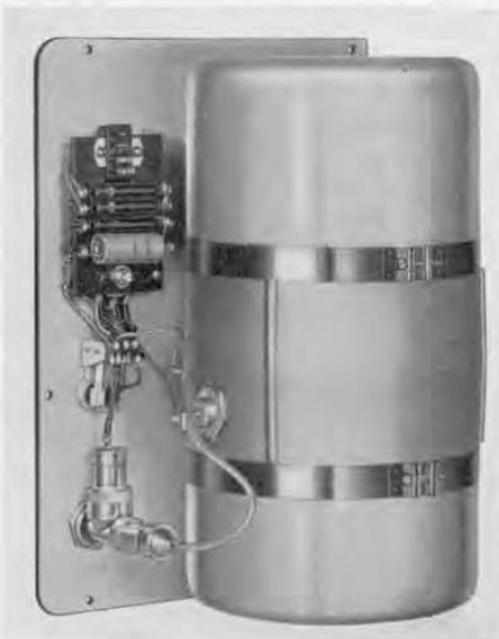
Figure 4. Rear view of the V-H-F Unit showing the casting that completely encloses the oscillator. Connections to the power supply unit are made through the connector at the upper right.
