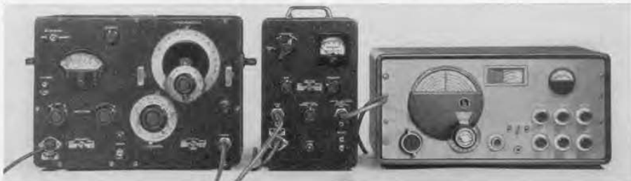
Figure 5. The Type 1021-AV V-H-F Standard-Signal Generator and the Type 1023-A Amplitude Modulator, arranged for tests on a communications-type receiver.
