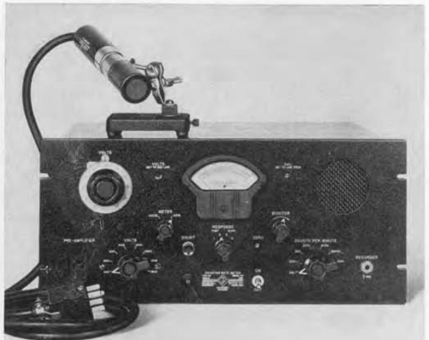
Figure 1. Panel view of Type 1500-B Counting-Rate Meter with counter tube and probe stand.
