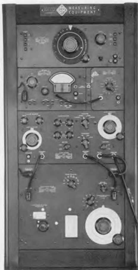
Figure 4. View of the Type 1610-A Capacitance Measuring Assembly consisting of guard circuit and bridge mounted in a relay-rack with associated equipment: Type 1302-A Oscillator, Type 1231-BRFA Amplifier and Null Detector, Type 716-P4R Guard Circuit, and Type 716-C Capacitance Bridge. Assembly includes relay rack and all necessary cables. Oscillator and amplifier operate from a 115-volt, 60 cycle power line.
