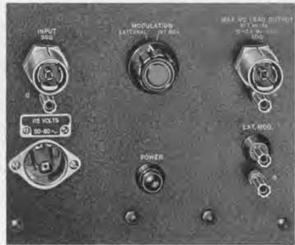
Figure 2. The Type 938-P Binding Post Assembly and the Type 874-P Panel Connector can be mounted as shown here on the Type 1023-A Amplitude Modulator to permit connection by either coaxial connector or double banana plug.
