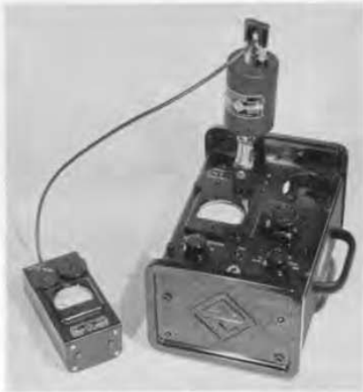
Figure 3. The Transistor Oscillator used as a tone source for the Type 1552-A Sound-Level Calibrator to standardize the Type 1551-A Sound-Level Meter.
