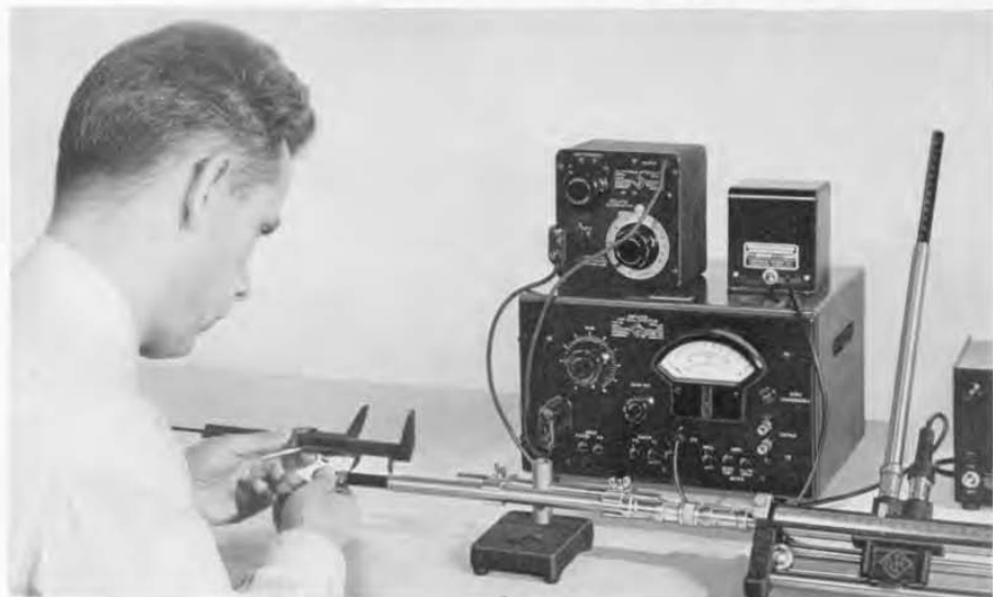
Figure 5. View of the slotted line and associated equipment set up for measuring VSWR of a pair of UG-type adaptors. The detector is a Type 1231-B Amplifier and Null Detector.
