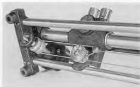
Figure 2. View of the drive mechanism showing the driving drum, ratchet take-up mechanism and nylon cord.
