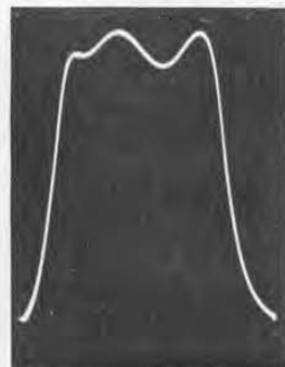
Figure 3. Oscillogram of the response characteristic of a filter as displayed by means of the arrangement of Figure 2.
