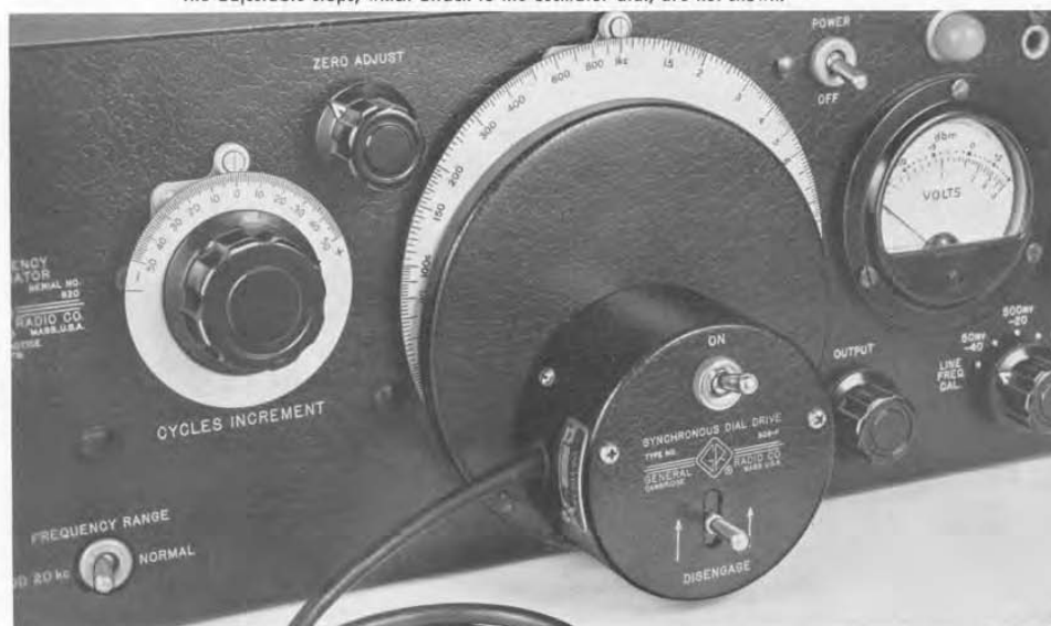
Figure 1. View of the Type 908-P2 Synchronous Dial Drive installed on a Type 1304-B Beat-Frequency Oscillator. The adjustable stops, which attach to the oscillator dial, are not shown.
