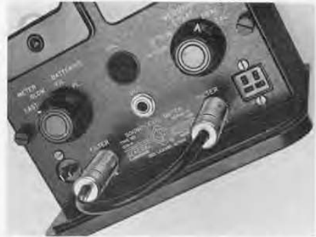
Figure 3. As shown here, the Type 1551-P11 20-db Pad plugs into jacks on the sound-level-meter panel.
