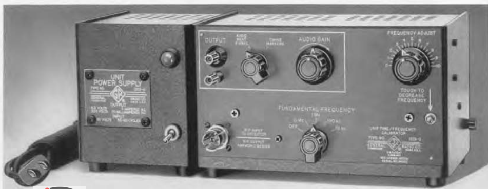
Figure 1. Panel view of the Type 1213-C Unit Time/Frequency Calibrator with Unit Power Supply.
