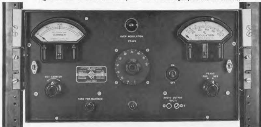
Figure 10. View of monitor with outer panel removed showing adjustments and controls.
