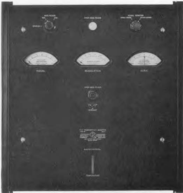
Panel view of the Type 1184-A-A Television Transmitter Monitor.
