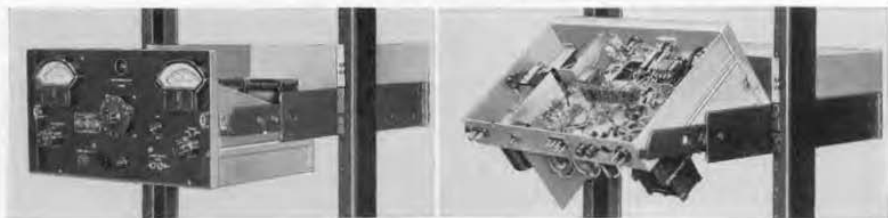
Figure 1. (Left) Type 1931-B Amplitude Modulation Monitor pulled forward on its slides. (Right) Tilted to expose underside of chassis.
