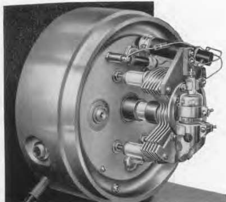
Figure 1. (Left) View of butterfly circuit in the Type 1209-B Unit Oscillator.
