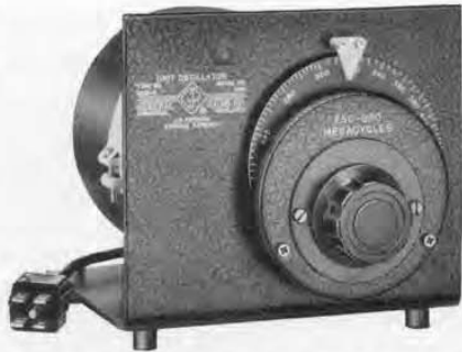
Figure 2. Panel view of the Type 1209-B Unit Oscillator. The new Type 1209-BL is identical in appearance except for the frequency calibration on the dial.
