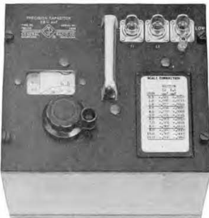
Figure 9. View of the Type 722-CD Three-Terminal Precision Capacitor. Outer conductors of Type B74 Coaxial Connectors provide the shield. Inner conductors are the capacitor terminals.
