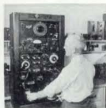
This scene in the General Radio Standards Laboratory shows the Type 1610-A Capacitance Measuring Assembly in use for the measurement of 3-terminal capacitors.
