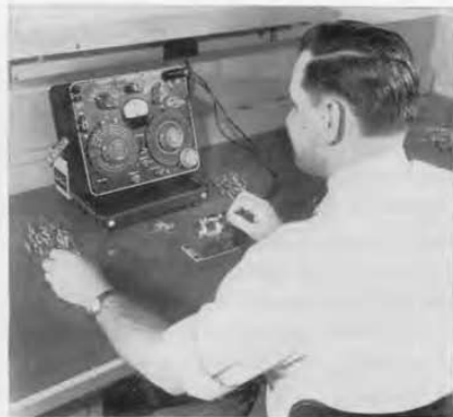
Figure 10. With the Test Jig, as shown here, the bridge can be set up for go-no-go testing to preset limits.
