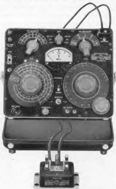
Figure 9. Bridge with Test Jig connected.
