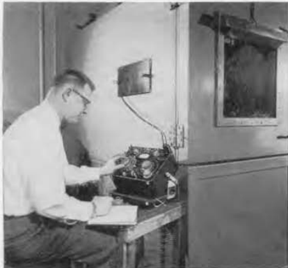
Figure 11. Bridge in use for 3-terminal measurements of sample in conditioning chamber.
