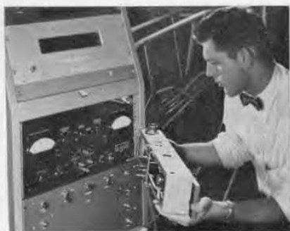
Figure 3. Inland Testing Laboratories use the Impedance Comparator in an automated instrumentation system for environmental reliability tests on capacitors.
