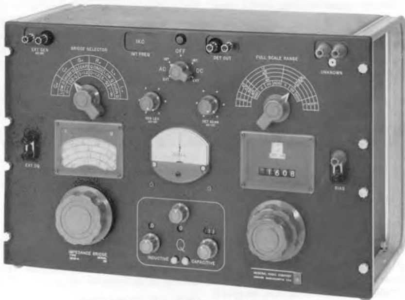
Figure 1. Panel view of the Type 1608-A Impedance Bridge.
