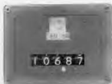
Figure 4. The digital CRL readout includes automatic decimal point location and illuminated indication of the units of measurement.
