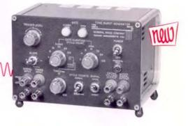
The Tone-Burst Generator is a unique instrument, which, when fed from an external oscillator, generates pulses, or bursts, of the input frequency. It is useful for testing the time response of ac circuits and for simulating the pulsed ac signals commonly used in audio and ultrasonic equipment, such as sonar.
