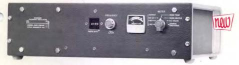
This new crystal oscillator combines high stability with the physical ruggedness necessary to withstand vibration and shock. It uses a 5-Mc, 5th-overtone crystal in an all-solid-state circuit of silicon transistors. Both crystal and circuit are held at constant temperature by a proportionally controlled oven. Fiberglas-epoxy etched circuits, cased transformers, and Mil grade electrolytic capacitors make the unit acceptable for many military and government applications.
