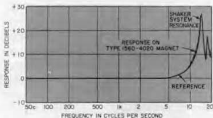
Figure 6. Response of Type 1560-P53 Vibration Pickup with and without magnetic clamp.
