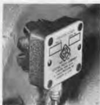
Figure 5. Vibration Pickup with Type 1560-P35 Permanent-Magnet Clamp.
