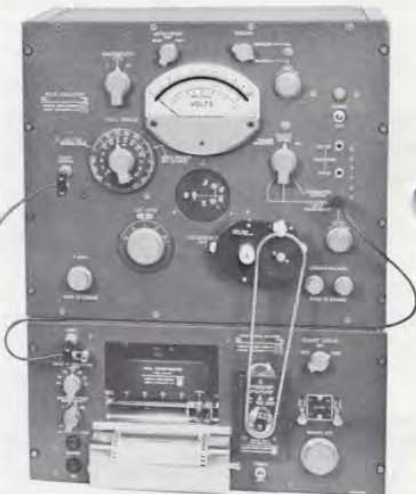
Figure 1. Type 1900-P3 Link Unit installed on the wave analyzer and graphic level recorder.
