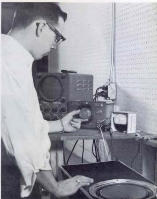
Figure 4. In a production test, the 1313 drives a loudspeaker over the entire audio range in one turn of the dial.
