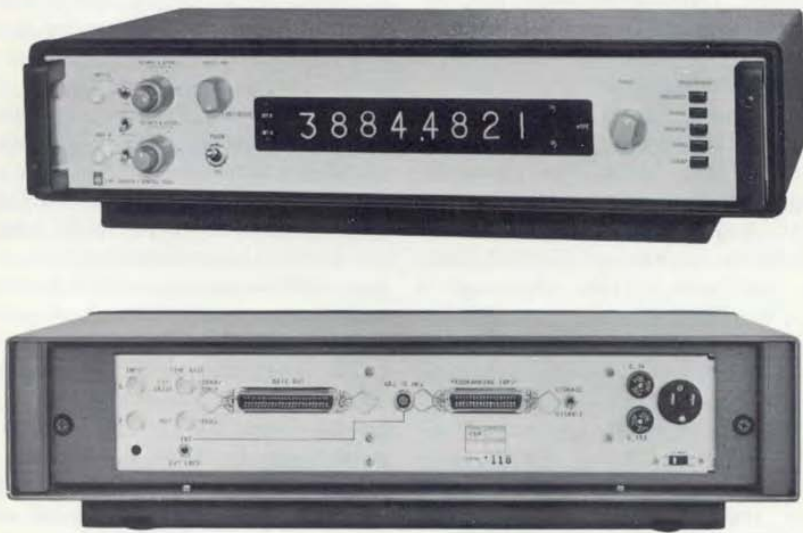
Figure 1. Type 1191 20-MHz Counter, front and rear panel views.
