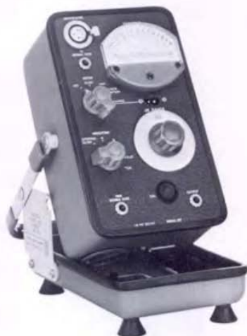
Figure 1. Precision sound-level meter, portable model.
